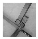
**STEP 4:** Take one support bar and put it in the outside of the upper frame and the inside of the bottom frame. Use two 2-3/8" D-Pins to lock it. Repeat this step on the other side.
