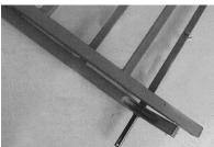
**STEP 3:** Open the upper frame and use two 2-3/8" D-Pins to lock the frame.
