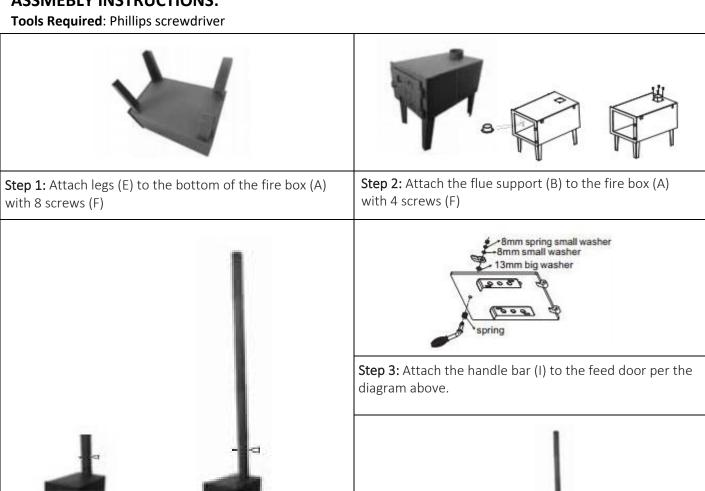
**Step 4**: Connect 3 pieces of flue pipe (C) to the top of the bottom flue pipe (K) and set all on the flue support (B). Then connect the top flue pipe (D) to the top of the flue stack (C).
