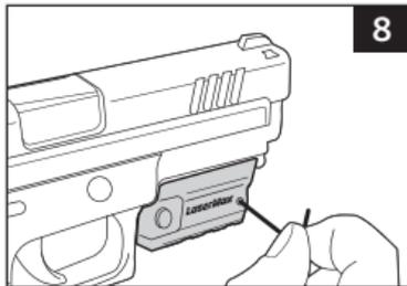
2. Windage adjustment: with the muzzle pointing forward and *adjustment tool* inserted into the *windage port*, a clockwise turn will shift the laser aiming point to the left and a counterclockwise turn will shift the laser beam to the right (figure 8).
