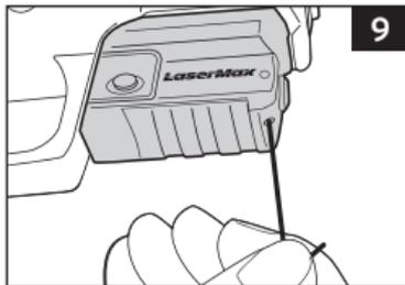
3. Elevation adjustment: with the muzzle pointing forward and *adjustment tool* inserted into the *elevation port*, a clockwise turn will shift the laser beam up and a counterclockwise turn will shift the laser beam down (figure 9).
