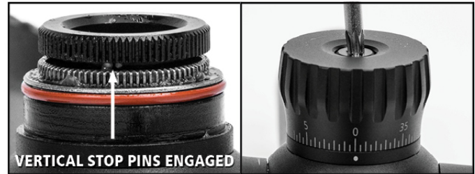
3b. Retighten the turret's top slotted screw.
