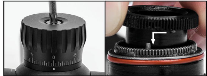
2g. Loosen the turret's top slotted screw. 3a. Position assembly's vertical stop pin against the turret's base vertical stop pin.
