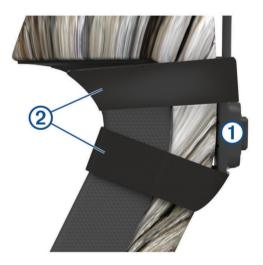
2 Secure the trigger to the bow using the included tape ②.
