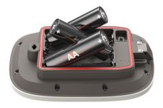
3 Replace the battery cover, and turn the D-ring clockwise.
