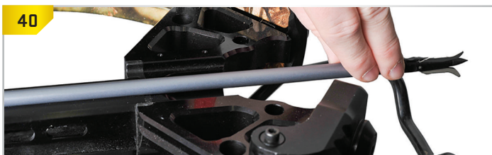
40 PROPER POSITION. Hold the arrow with your index and middle finger and your thumb just behind the broadhead.
