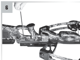
Remove stock screws.
