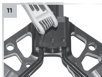
Remove 1/4-inch setscrews holding foot stirrup in place.
