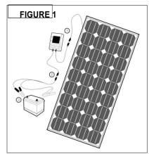
When installing solar panels configuration and systems, please carefully observe correct cable connections and polarity. The solar panels can be damaged by not observing the correct electrical installation and polarity; in addition, this will void the warranty of your solar panels. Having a multimeter handy will help to confirm correct polarities.
