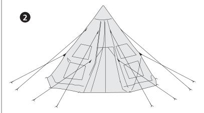
From inside of the tent, insert the small end of the top of the pole into the center of the roof. Stand the pole vertically with the pole stabilizer in the middle of the floor. Have another person hold the pole in place, and begin to stake down the guy ropes. It is recommended to stake down the ropes in a star-type pattern to keep a uniform balance of the tent. Adjust and secure the tent's floor stakes to make the tent taunt. (pic. 2)
