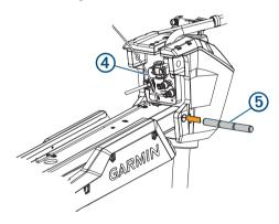
5 While lifting up on the steering system housing, push the pivot pin (5) through the housing and the mount to hold it in place.
