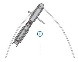
You must install the mount with the bumper ② overhanging the gunwale of the boat.
