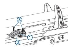
You may need to lift up the mount and flip over the gas spring if it was positioned on the other side of the mount during the previous installation steps.
