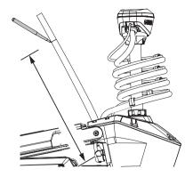
2 With the motor in the deployed position, route the transducer cable through the channel along the right (starboard) side of the mount (1).
