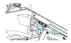
2 Push the connector onto the port on the display panel, and rotate the locking ring clockwise to secure it.
