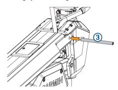
6 Using a 4 mm hex bit or hex wrench, secure the pin using the screws and washers (4) on both sides.
