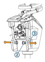
4 Holding the pull cable 4 up, place the steering system housing onto the lower half of the mount, aligning the lower holes on the housing with the holes on the mount.
