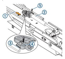
2 If necessary, pivot the upper gas spring ② toward the bottom of the mount so the base of the gas spring aligns with the safety rod and mounting holes.
