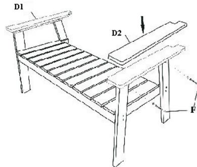
**STEP 3:** Attach the Back (E) to Back Legs (C) with two Short Bolt, Nut and Washer Sets (F) and to Armrests (D) with two Long Bolt, Nut, Washer Sets (G) using a Philips screwdriver (not included).
