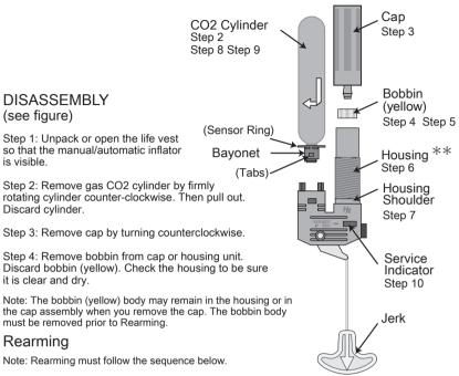
Step 5: A new bobbin must be used. New bobbin must have been purchased within three (3) years. If bobbin purchase date is unknown, check date on bobbin, replace if over three (3) years.
