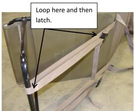
Finished blind shown below. The straps holding the support bar will also adjust the backrest angle.
