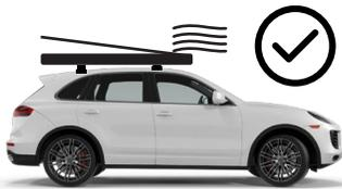
Place the tent opening side towards the back to prevent accidental openings from the wind, and to minimize drag.
