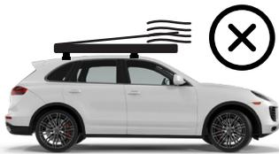
Make sure to always secure the locks to prevent air to get in the tent while driving. Never place the tent with the opening side against the drag.
