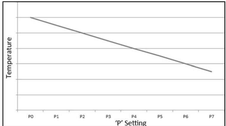
Increasing the 'P' value decreases the fuel feed rate, resulting in lowering the Grill temperature. Adjust the 'P' setting for the desired temperature and/or smoke output. **For trouble free cooking, P2 is the recommended setting.**
