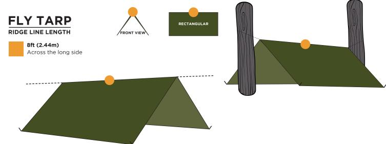
This pitch provides an asymmetric shelter for more equalised storm protection when the wind is variable.
