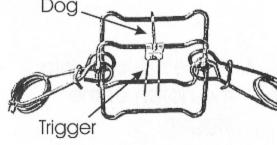
Place the dog into the notch of the trigger.
