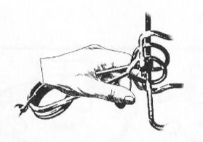
Extend spring away from the rotating jaws of the trap. Then with one hand, compress the spring.
