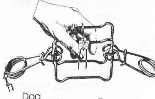
While the springs are compressed, bring the trap jaws together.
