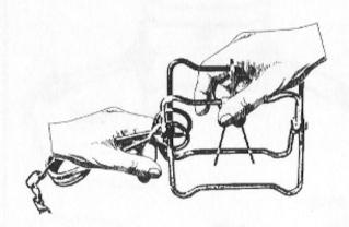
While keeping the spring compressed, bring the trap jaws together.
