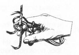
Extend both springs away from the rotating jaws of the trap.
