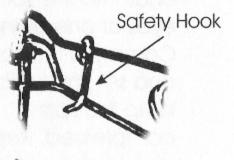
Grip and compress one spring and set safety hook to keep the spring compressed. Repeat step for the opposite spring.
