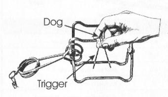
Place the dog into the notch of the trigger.
